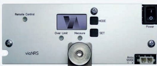
Control panel in the battery housing.
