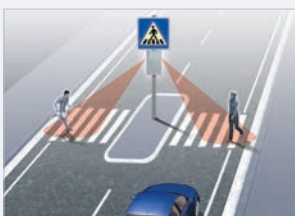
viafalcon PCD-2: Two independent detection zones allow the simultaneous observation of two crossings from a middle reservation (180°).
