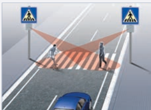
viafalcon PCD-1: The single forward detection zone allows the observation of pedestrian crossings from the pavement. Warning signs can be switched on or green light phases can be extended.
